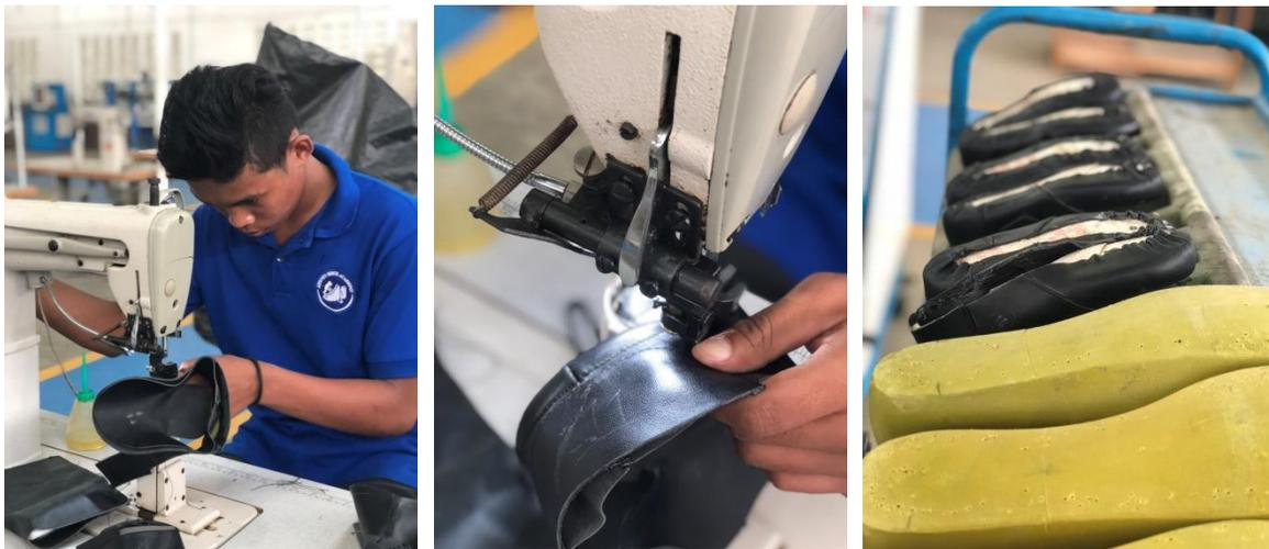
*Victor Cawayan (left) stitches his pattern into shoe uppers (center). The shoe uppers are then nailed to lasts (right) for them to assume the shape and form of a shoe.*
